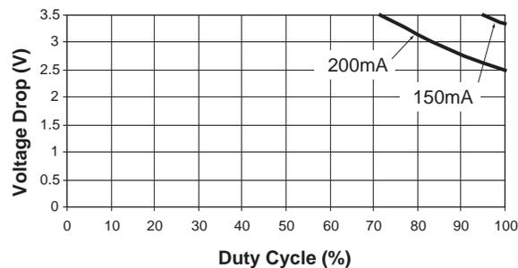
**Device Duty Cycle vs.  $V_{DROP}$**
